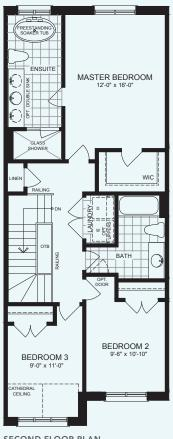
SECOND FLOOR PLAN ELEVATION A2
